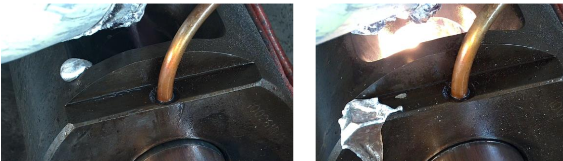
Figure 1: Pouring process without (left) and with (right) lubricant combustion in the shot sleeve
